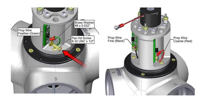
h. Fit and connect feather link wire to micro-switch mount assembly. Connect motor wires.
