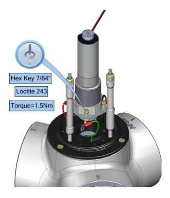
d. Attach micro-switch mount assembly (note orientation) to motor mount plate.
