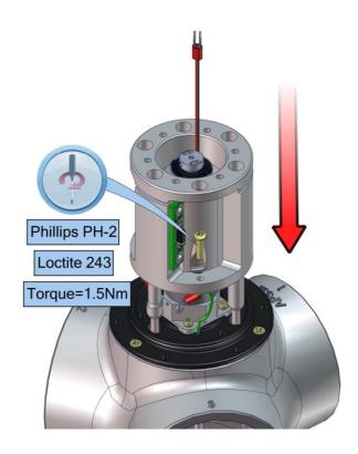
e. Place the PC Brake Cover onto the motor. Ensure that the wires align with the slot. Push on until the cover seats on top of the motor.
