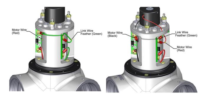
i. Secure PC motor lead wires with heat shrink to keep motor wires clear of pitch change limit rods.
