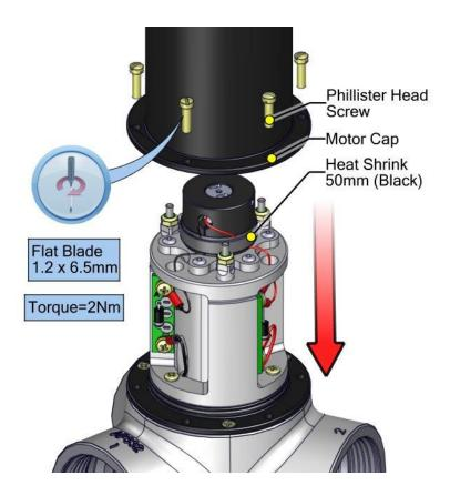
j. Test hub assembly for correct operation
